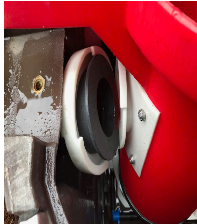
Overflow disconnected from carriage
