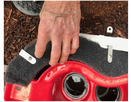
STEP 5: Remove poly-mat, overflow flush tubes and filter baskets.
